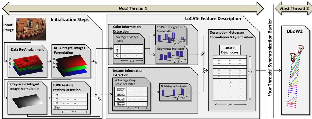
Figure 5. The GPGPU based pipeline of the proposed vPR system. The approach can be divided into three main processing components: (Left) the initialization steps, (Middle) the LoCATE descriptors calculation and (Right) the loop closure detection algorithm.
