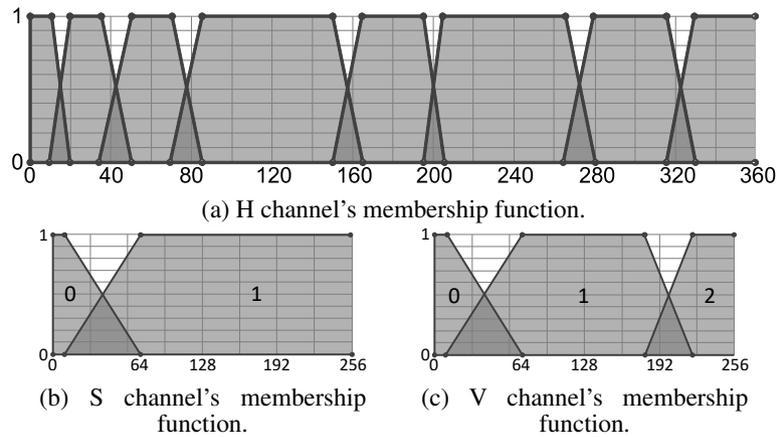
Figure 2. Membership functions used in the first stage of the fuzzy system [34].
